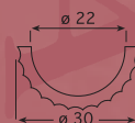
C COL3325 H.Q. Mezzo tronco rigato Ø 30 x 15 x h. 305 cm Half Fluted pillar 11 13 / 16 " x 5 14 / 16 " x h. 120 1 / 16 "
